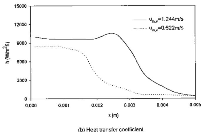
Figure 8. Effect of vapor inlet velocity on condensation in miniature tubes ( $\dot{m}_i = 10^{-5}kg/s$ ,  $T_{sat} = 363K$ ,  $T_w = 340K$ )
