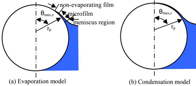
Fig. 2 Evaporation and condensation occurred on sintered particles
