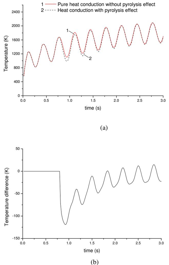
**Figure 5** Temperature transients at the laser spot center on the front surface for  $q_0'' = 150 \text{ W/cm}^2$ . (a) comparison of the results with and without pyrolysis effect. Curve 1: Pure heat conduction without pyrolysis effect. Curve 2: Heat conduction with pyrolysis effect. (b) difference between the results with and without pyrolysis effect (Curve 2 minus Curve 1).
