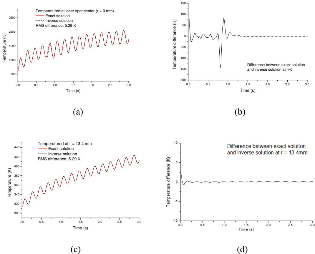
**Figure 12** Recovered front surface temperature for  $f = 5$  Hz. (a) comparison of exact solution and inverse solution at the laser spot center; (b) difference between the exact solution and inverse solution at the laser spot center (inverse solution minus exact solution); (c) comparison of exact solution and inverse solution at the radius of 13.4 mm; (d) difference between the exact solution and inverse solution at the radius of 13.4 mm (inverse solution minus exact solution).
