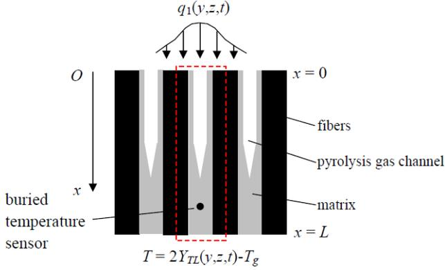
**Figure 2** Physical model of 1-D gas flow channels.
