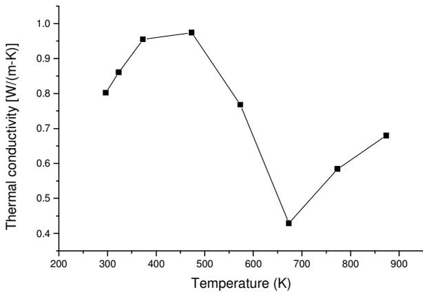
**Figure 4** Thermal conductivity of carbon/epoxy composite [3].
