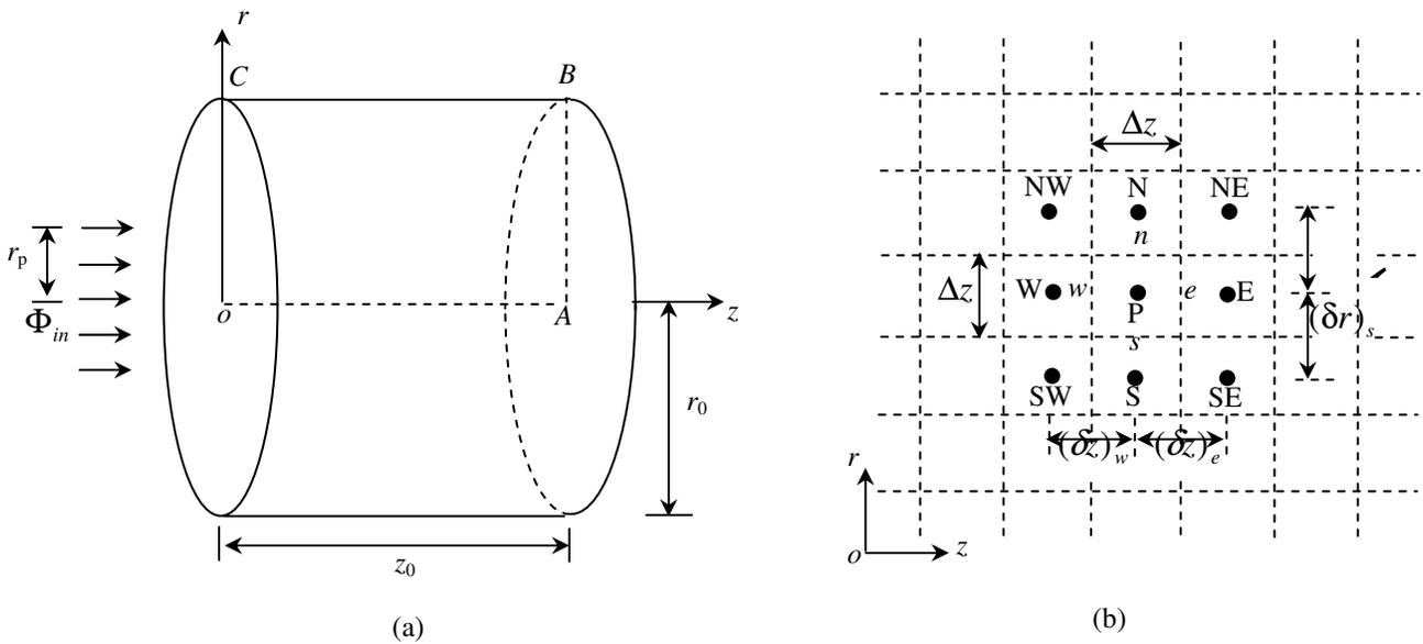
Figure 2 Physical model and grid system for 2-D analysis
