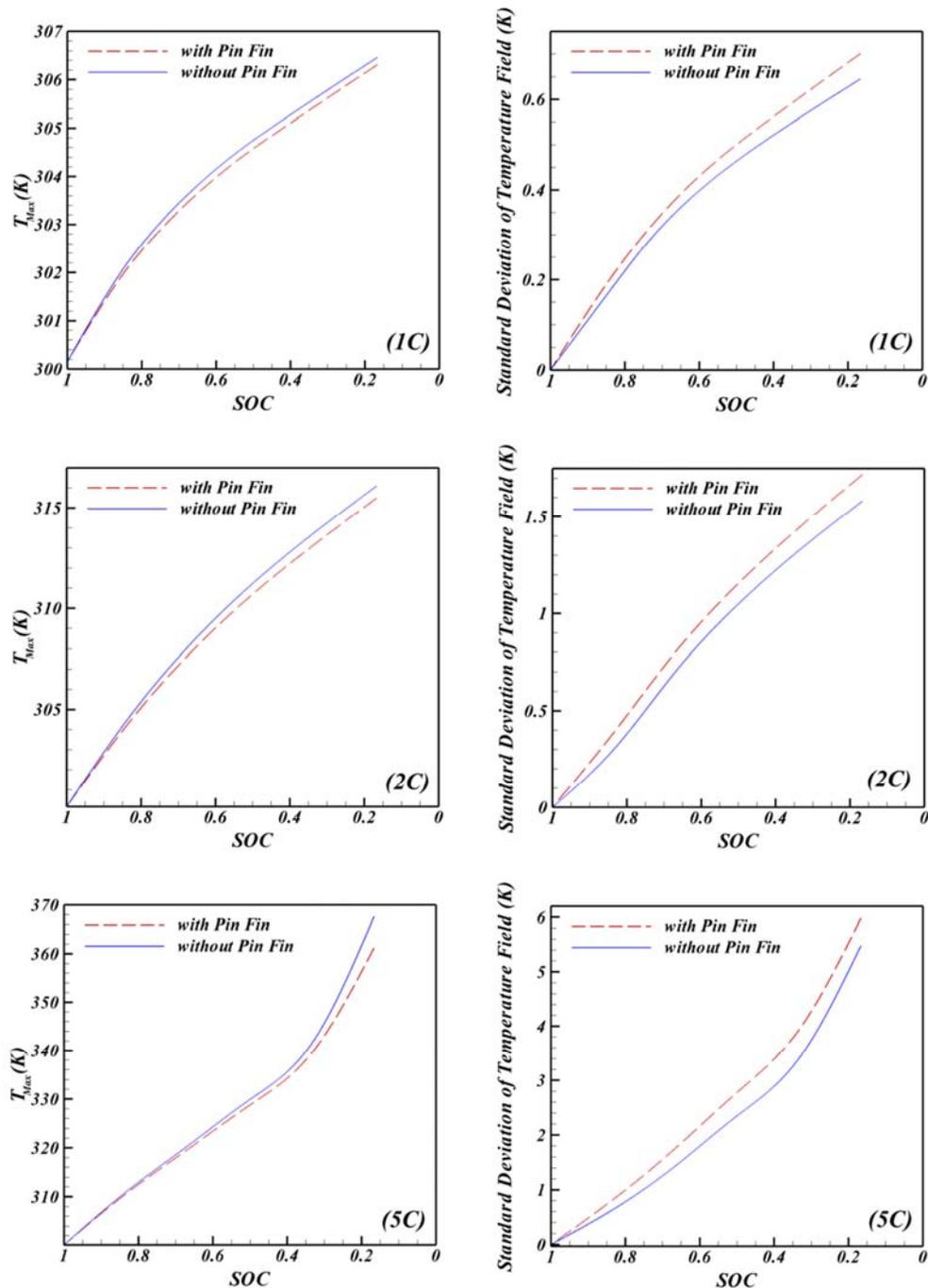
Fig. 4 Maximum temperature inside the battery and standard deviation of temperature field versus SOC
