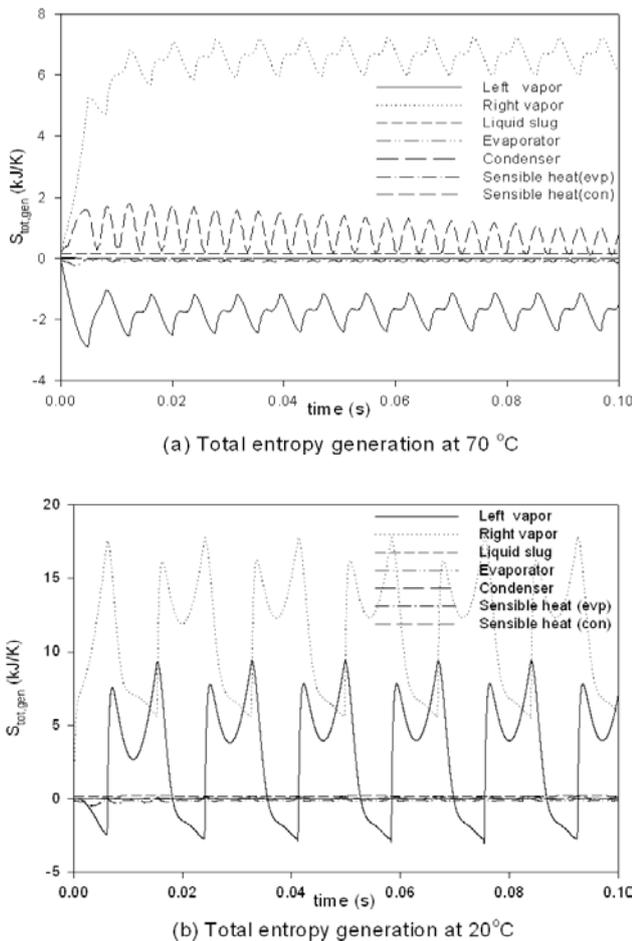
Figure 2. Total entropy generation at different initial temperatures
