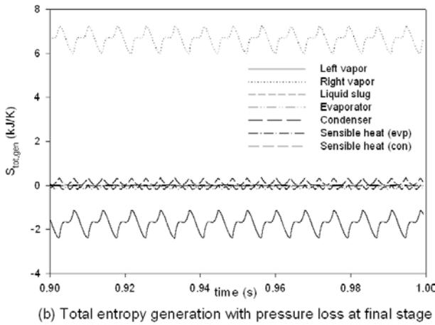
Figure 3. Total entropy generation with or without pressure loss at bend
