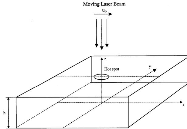
**Figure 7** Physical model of Laser Chemical Vapor Deposition (Zhang, 2003)
