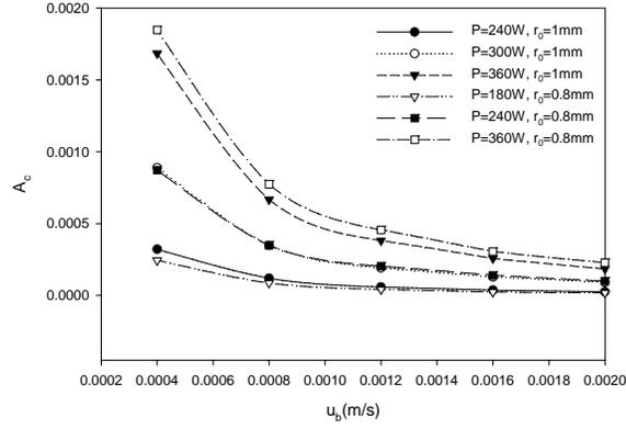
**Figure 10** Dimensionless cross-sectional area vs. scanning velocity (Zhang, 2004).
