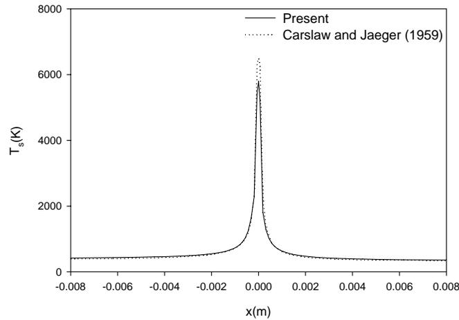
**Figure 8** Comparison between analytical and numerical solutions for pure conduction
