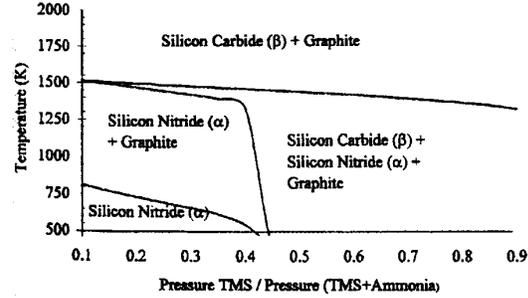
**Figure 6** Deposition map for mixture of TMS and  $\text{NH}_3$  at 0.5 atm and at thermodynamic equilibrium (Jakubenas et al., 1998)
