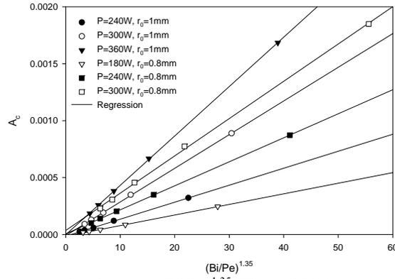
**Figure 11** Dimensionless cross-sectional area vs.  $(Bi/Pe)^{1.35}$  (Zhang, 2004).
