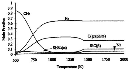
**Figure 5** Composition vs. temperature for a 1:1 mixture of TMS and  $\text{NH}_3$  at 0.5 atm and at thermodynamic equilibrium (Jakubenas et al., 1998)
