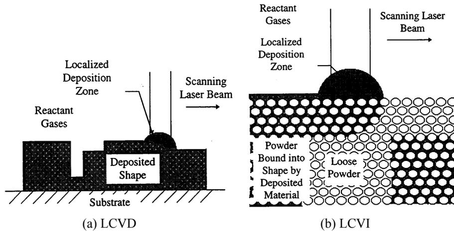
**Figure 1** Schematic of SALD and SALDVI (Jakubenas *et al.*, 1997).
