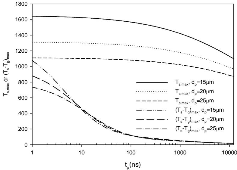
**Figure 13** Maximum powder temperature and maximum temperature difference vs. pulse width ( $J = 1.25 \times 10^5 \text{ J/m}^2$ ; Zhang, 2006)
